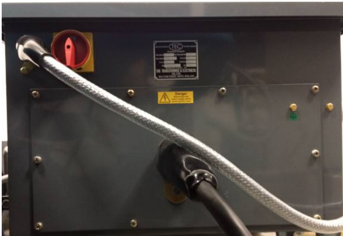
Switch OFF AFC-11 Goniometer controller.
