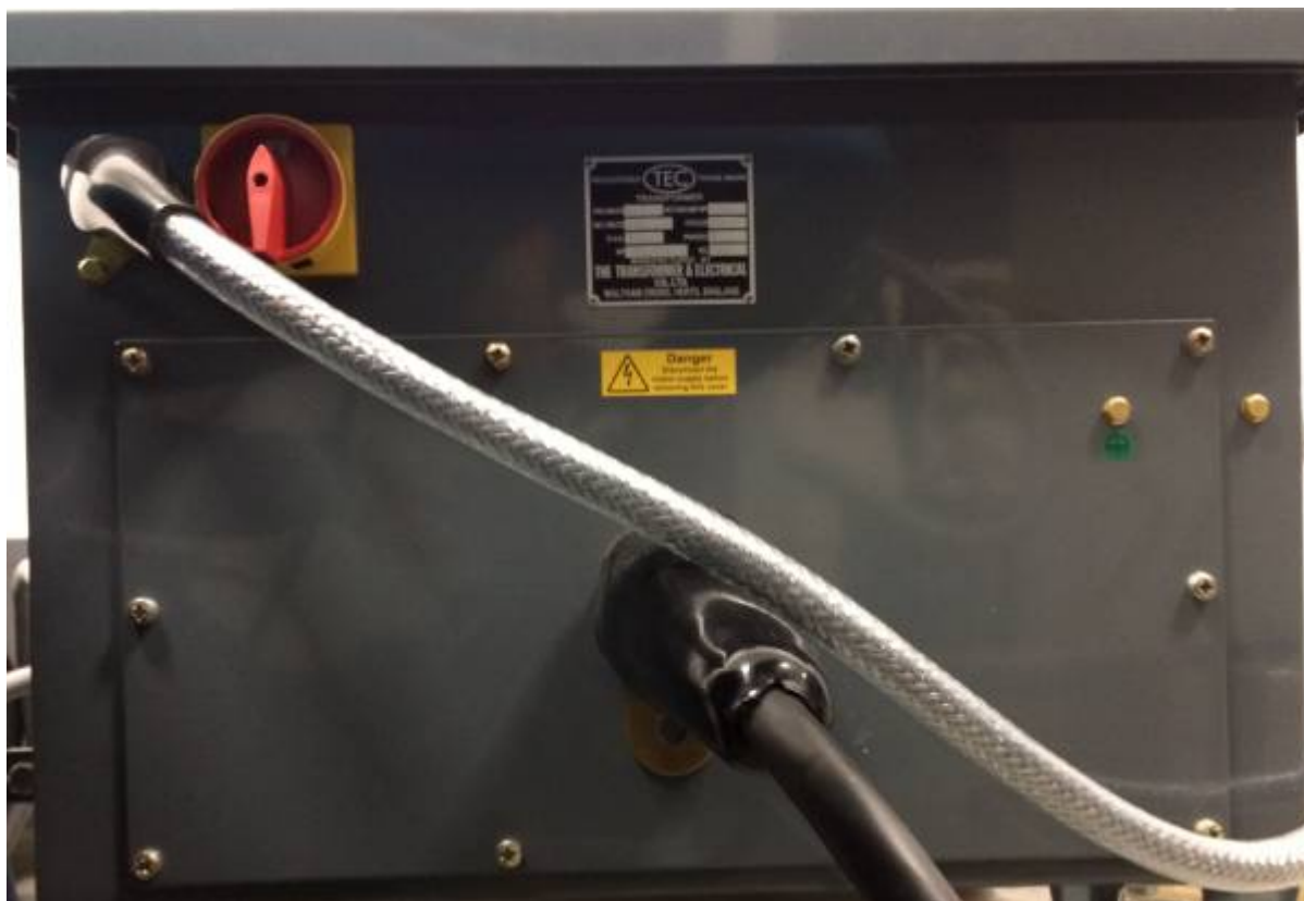
Switch OFF AFC-11 Goniometer controller.
